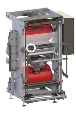
Triggers the mainframe nip to clamp and hold the web in the event of web break due to an improperly prepared splice
